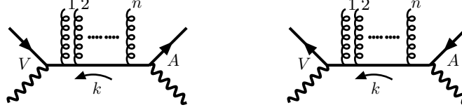
Fig. 5.2. Compton scattering amplitude in the external color field
